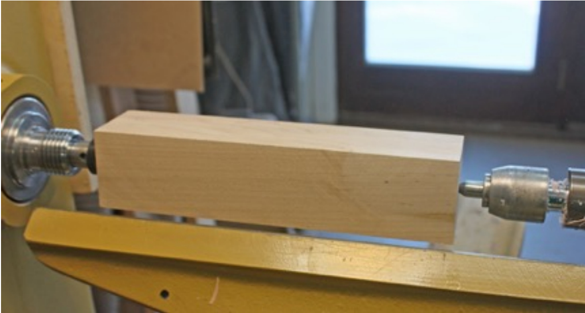
1. Blank mounted between centers
