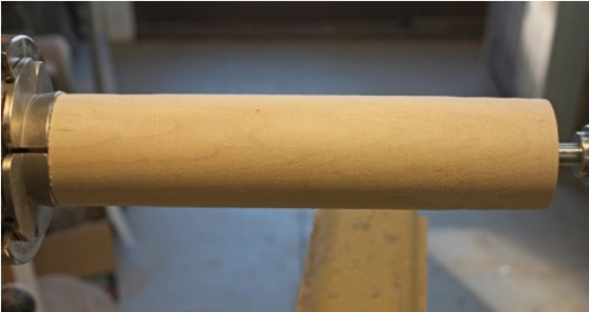
3. blank mounted in 4 jaw chuck
