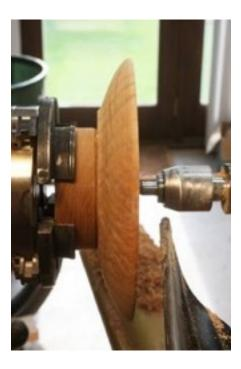
Here I've roughed out the outside of the vessel, up the point where it reaches the mounting block.
