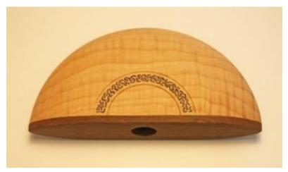
The top has been glued to the vessel and the edges sanded smooth. It's important to not sand too aggressively and sand away any details. The base is held to the vessel with a 1/8" brass pin epoxied in holes drilled in both the base and the center of the vessel. To find the center, I wrap a cloth tape measure around the outside curve of the vessel and divide the measurement by 2.
