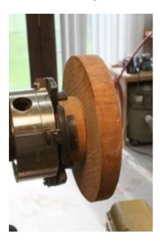
This is a side view of the blank mounted on the lathe. It's important to note that the side of the blank facing the headstock will become the outside of the vessel, the opposite of the way you normally turn a bowl.
