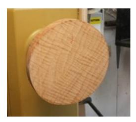
The blank has been mounted to the lathe. In this case, I'm using a solid piece of wood rather than gluing together 2 separate pieces. I've used double sided turners' tape to attach the blank to a waste block. This allows me to use the
